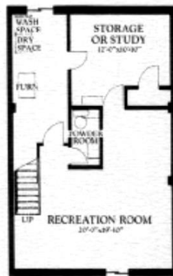
OPTIONAL FINISHED BASEMENT Front Recreation Room Non-Walkout
